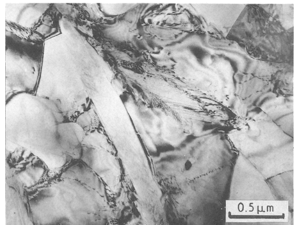
Figure 8 Characteristic subgrain structure in deformed SiC_w/Al-Mg composite.
