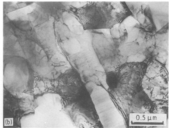
Figure 7 (a) Random dislocation tangle in as-cast SiC_w/Al-Cu composite. (b) Dislocations arranged in well-defined subgrains in as-cast SiC_w/Al-Si composite.
